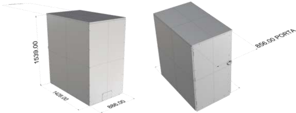
Figure 8: Cargo Box: Sketch and Dimensions
